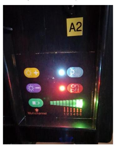
To change a channel, hold down the green multi-channel button for at least 5 seconds until the green bars flash on the current channel setting. Keep tapping the channel button until the single green light changes to the channel you want. After a couple of seconds, it will stop flashing and settle on the channel number.
