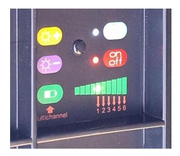
This timing light is now set to channel 1. If operating as one field of play, with multiple timing lights, the lights must all be on the same channel. If it works fine on channel 6 there is no need to change the channel.
