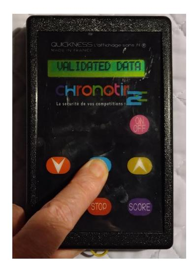
5: If using double detail use the Down arrow to cycle through AB/CD etc (only shows on timing clocks, not on the controller
