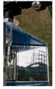
Looking from the archer's position, the clear glass has the 5 x 3 grid pattern, behind the glass there is the mirror which has a horizontal line and three vertical lines.
